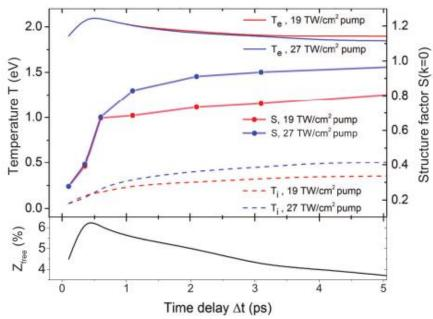
Ultrafast heating in cryogenic hydrogen by free electron laser x-ray burst.
