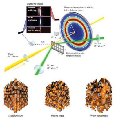
Upper: Schematic of MEC instrument at LCLS; 50 fs monoenergetic X-ray beam hits Al target.
